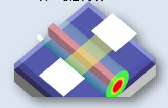
Phase modulator:  $V_{\pi}L\alpha = 14 \text{ dBV}$
